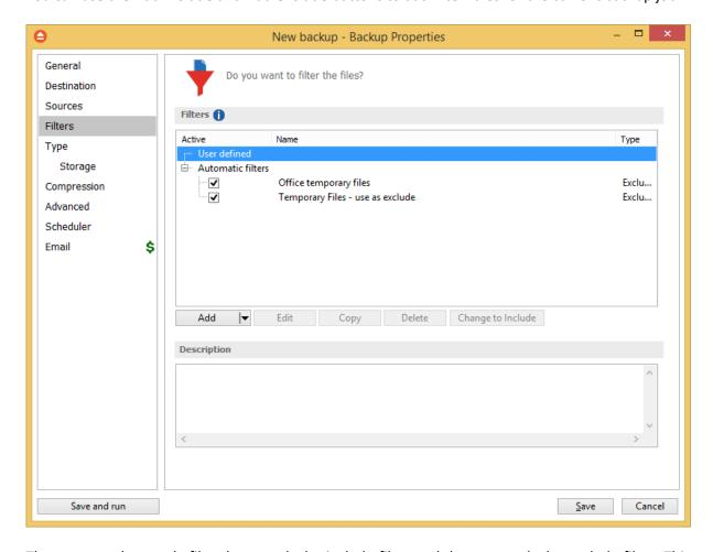
The system selects only files that match the include filter and do not match the exclude filter. This means the exclude filter is more powerful: if a file satisfies both include and exclude filters, it will be excluded.
